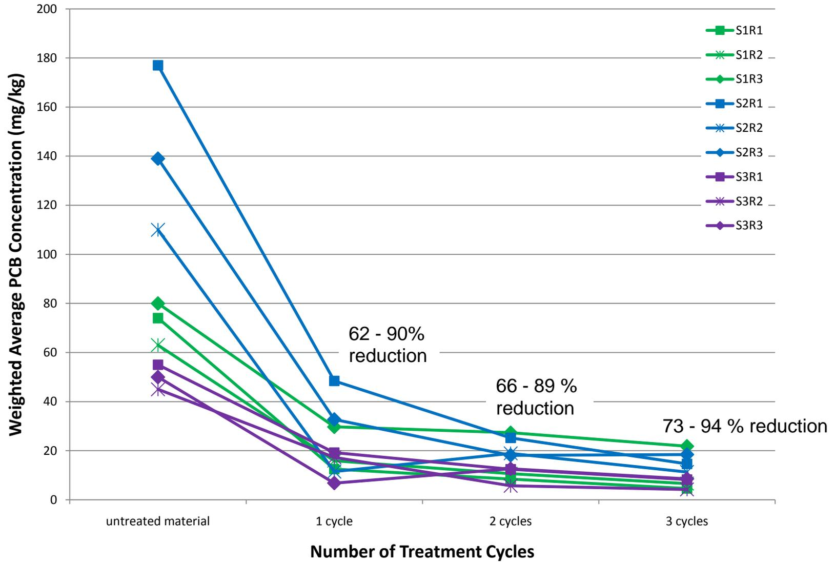
**Figure P-2 - Average PCB\* Concentrations of Bench Scale Inputs and Outputs
